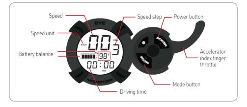
1) Speed step setting Can adjust with 🚺 button.
